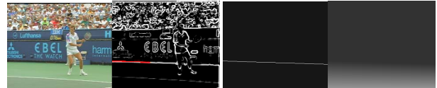
Fig. 4. Processed image in DGP module, from left to right, Stefan sequence, image after edge filter and line detection (red), dominate line, and depth map
